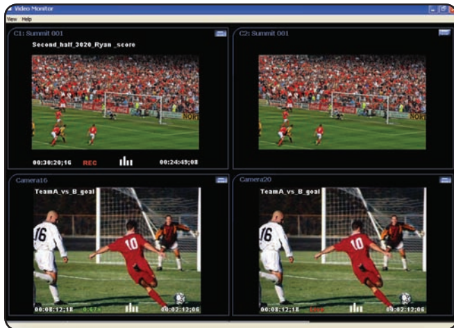
Internal multiviewer output on VGA provides a quad split display of the all channels in real time (Requires optional AppCenterPro).
